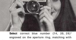
quide number of flash unit. With flash unit, set shutter speed at 1/30 sec. With electronic flash unit, any shutter speed
